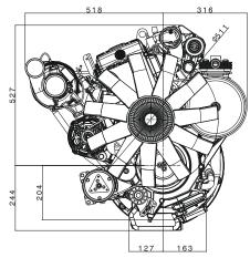
Standard base engine for 23° inclined installation with full equipped FEAD and transmission interface for Allison S1000 / S2000 / S2500 series. Limited flexibility for FEAD aggregates and transmissions.
