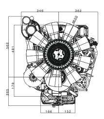
Standard base engine for vertical installation with full equipped FEAD and transmission interface for ZF8HP90 or Allison S1000 / S2000 / S2500 series. Deep Fording and EMC mil.461-E upgrade potential.
