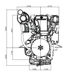
Standard base engine for vertical installation with full flexibility for customer specific FEAD and transmission interface. Deep Fording and EMV mil.461-E upgrade potential.
