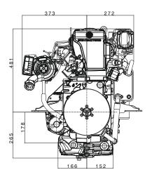
Standard base engine for vertical installation with full flexibility for customer specific FEAD and transmission interface.
