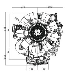
Standard base engine for vertical installation with full equipped FEAD and transmission interface for ZF8HP90 or Allison S1000 / S2000 / S2500 series. Deep Fording and EMC mil.461-E upgrade potential.
