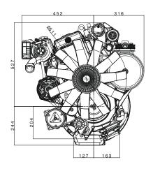
Standard base engine for 23° inclined installation with full equipped FEAD and transmission interface for Allison S1000 / S2000 / S2500 series. Limited flexibility for FEAD aggregates and transmissions.
