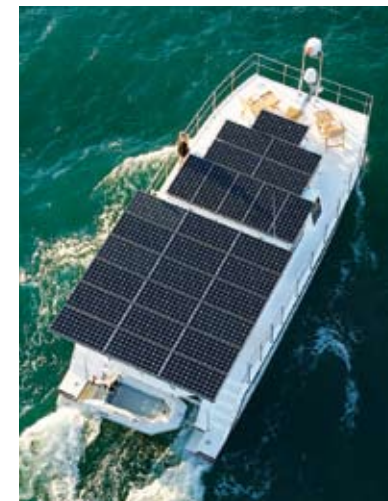
LOOKING UP. The solar panels on the roof provide enough power to run the boat.
